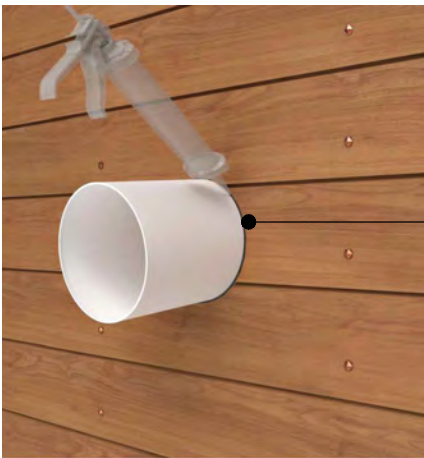
Continuous weather seal around pipe
